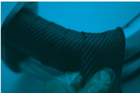
3. As a final step the clamps (provided in the kit) must be mounted to each end of the exhaust pipe, to fasten the wrap; if there are very accentuated curves it is preferable to insert the clamps also on them.
